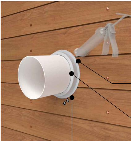
No sealant to drain
