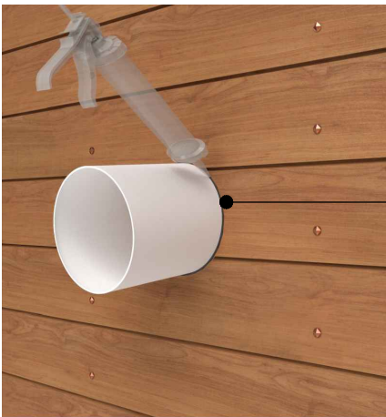
Continuous weather seal around pipe
