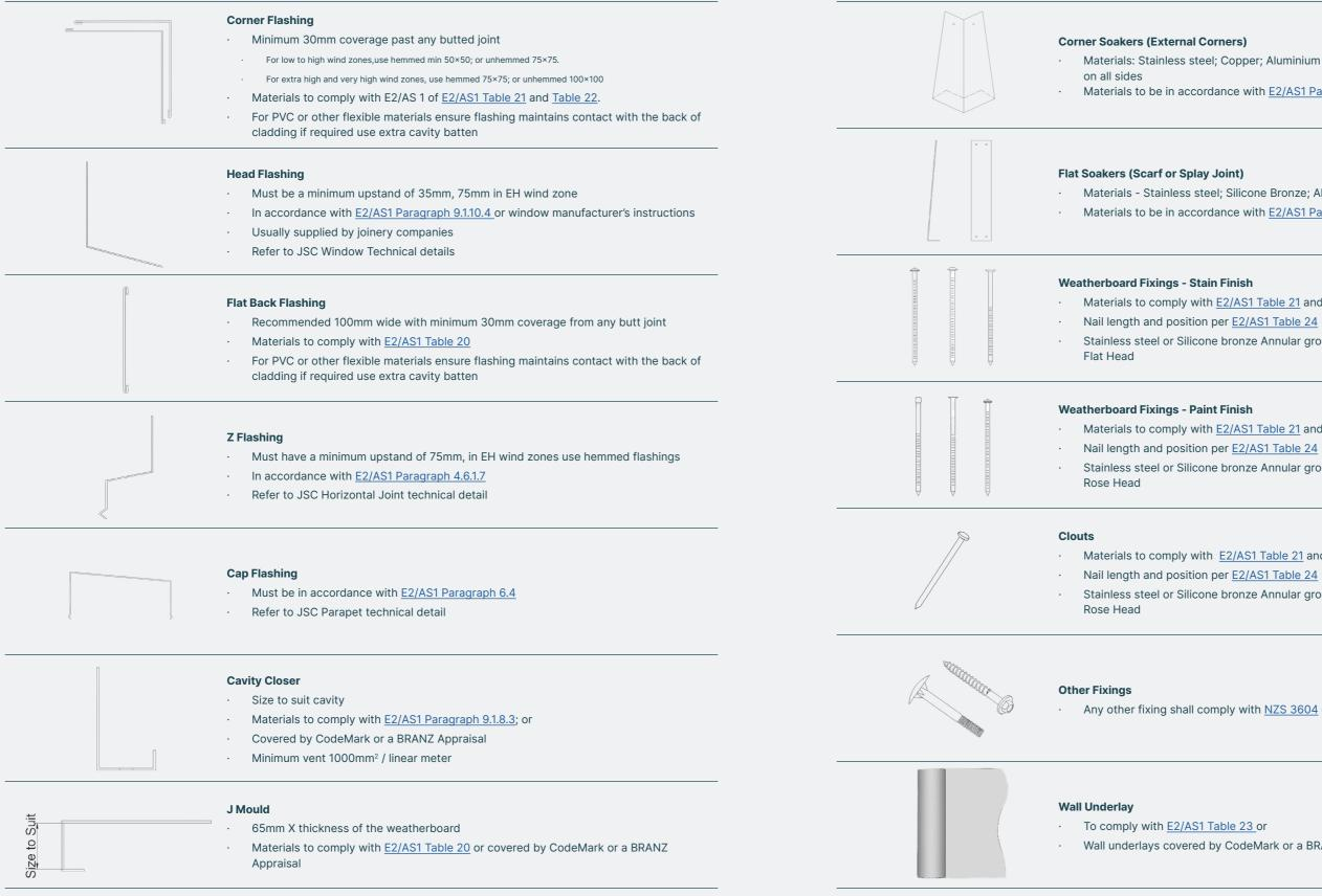
Materials: Stainless steel; Copper; Aluminium + Powder Coated; Galvanized + Painted
