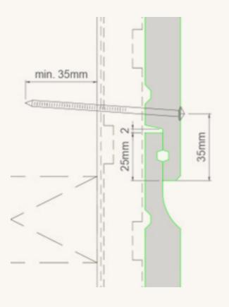
Figure 1 - Typical Vertical Shiplap Weatherboard Installation
