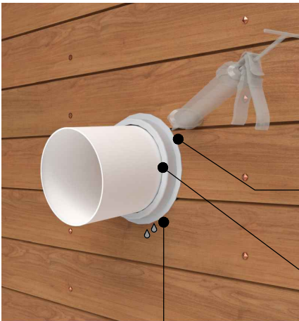
No sealant to drain
