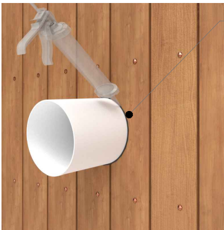
Continuous weather seal around pipe
