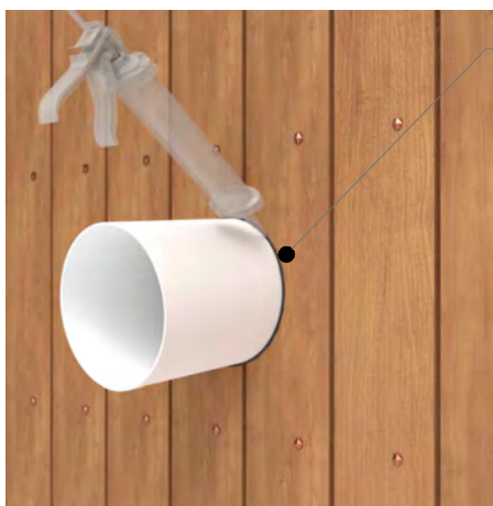
Continuous weather seal around pipe
