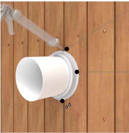
No sealant to drain
