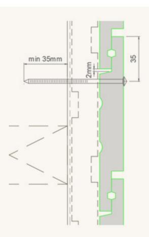
Figure 1 - Typical Vertical Shiplap Weatherboard Installation
