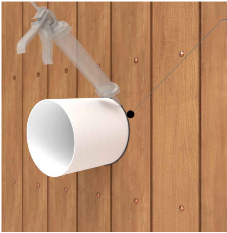
Continuous weather seal around pipe
