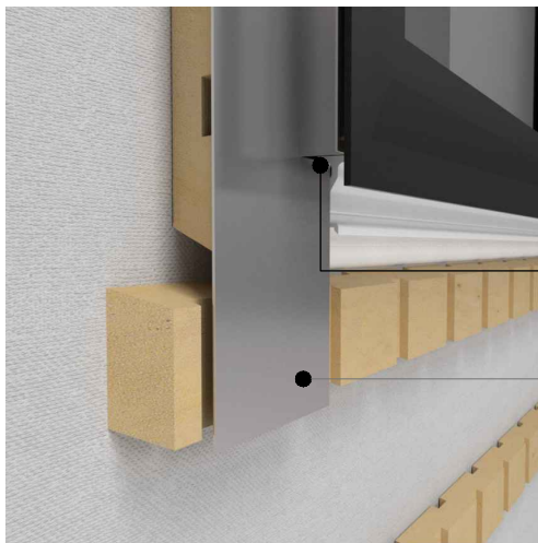
Cut and fold J Mould J Mould to extend past sill cavity batten
