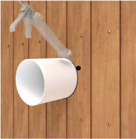
Continuous weather seal around pipe
